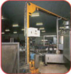
CAP / CROWN CORK ELEVATOR
