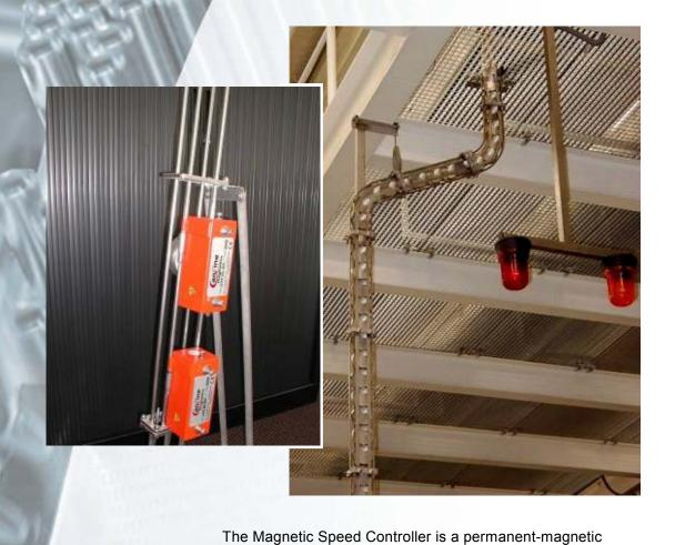
solution to control the speed of your aluminium cups and cans for all kinds of occasions and applications during your production process. The working principle of the controller is based on eddy currents. Eddy current controllers do not have any mechanical contact with moving parts and thus no wear and tear of it.
