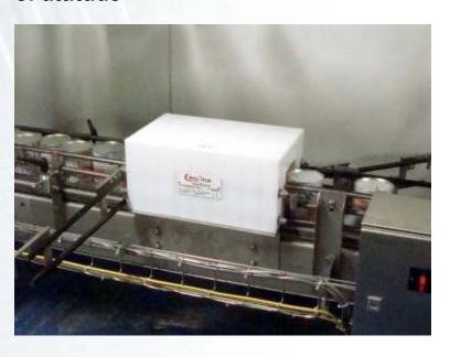
The high speed, inline Twister from CANLINE Systems gently and rapidly inverts or rotationally positions your cans, jars, bottles, ampoules, boxes and other containers towards any angle you want within a 450 mm length. The Twister inverts your product in a continuous flow in filling and packaging operations.
