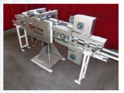
CANLINE Systems introduces a completely new magnetic upender for (can) bodies coming out of a welding unit into a 3piece can production line.
